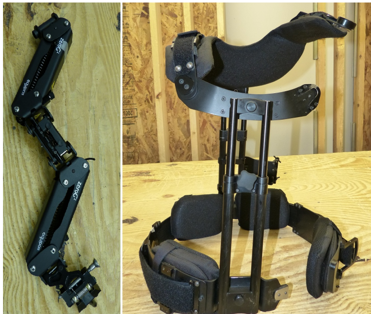
Figure 5. Equipois zeroG2 arm (left) and Exo vest (right).
