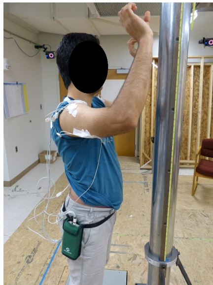
Figure 8. Reference contraction posture, during which EMG measures were obtained for purposes of normalization.
