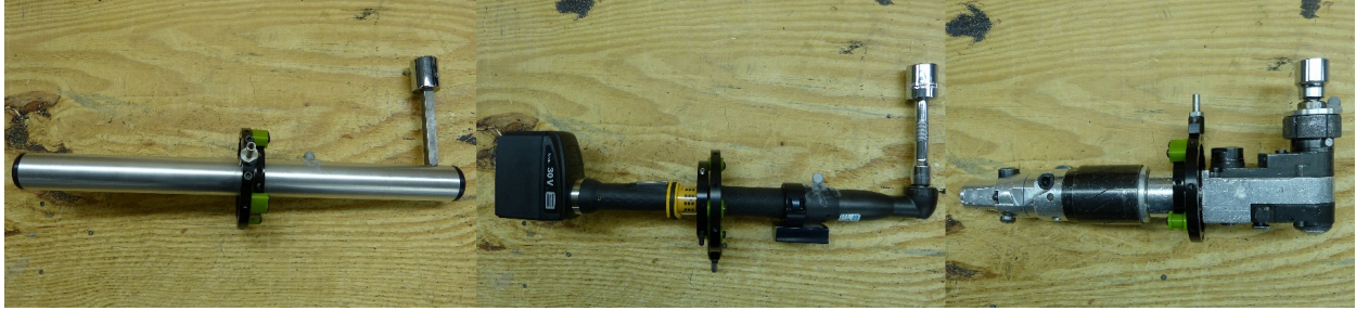
Figure 6. Three hand tool differing in mass (1.1, 3.4, and 8.1 kg, from left to right).
