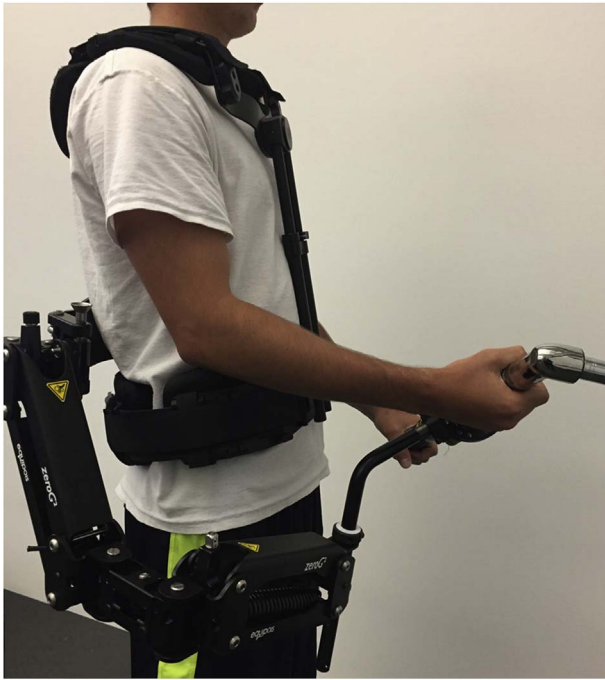
Fig. 1. Sample of the Steadicam Fawcett Exoskeletal vest attached to an Equipois mechanical arm. The vest and arm were used together to support the weight of nutrunner (shown) and impact wrench hand tools.
